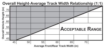
The measurements are to be taken from the ground to the tallest point of the vehicle for the Overall Vehicle Height and the normal track measurement as stated in Section 12 for the Average Track Width. (See figure on next page.)
